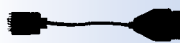
BMW-OBD II 16-pin Vehicle Adapter (for the 3596E Oil Reset Tools only)
