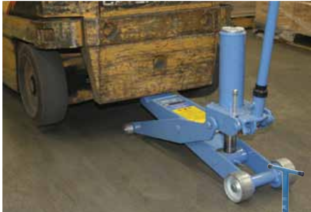
Polyamide wheels are superior to cast wheels due to their high mechanical strength and durability.
